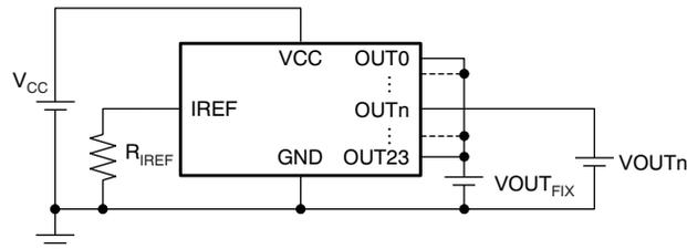
Figure 6. Constant Current Test Circuit for OUTn
