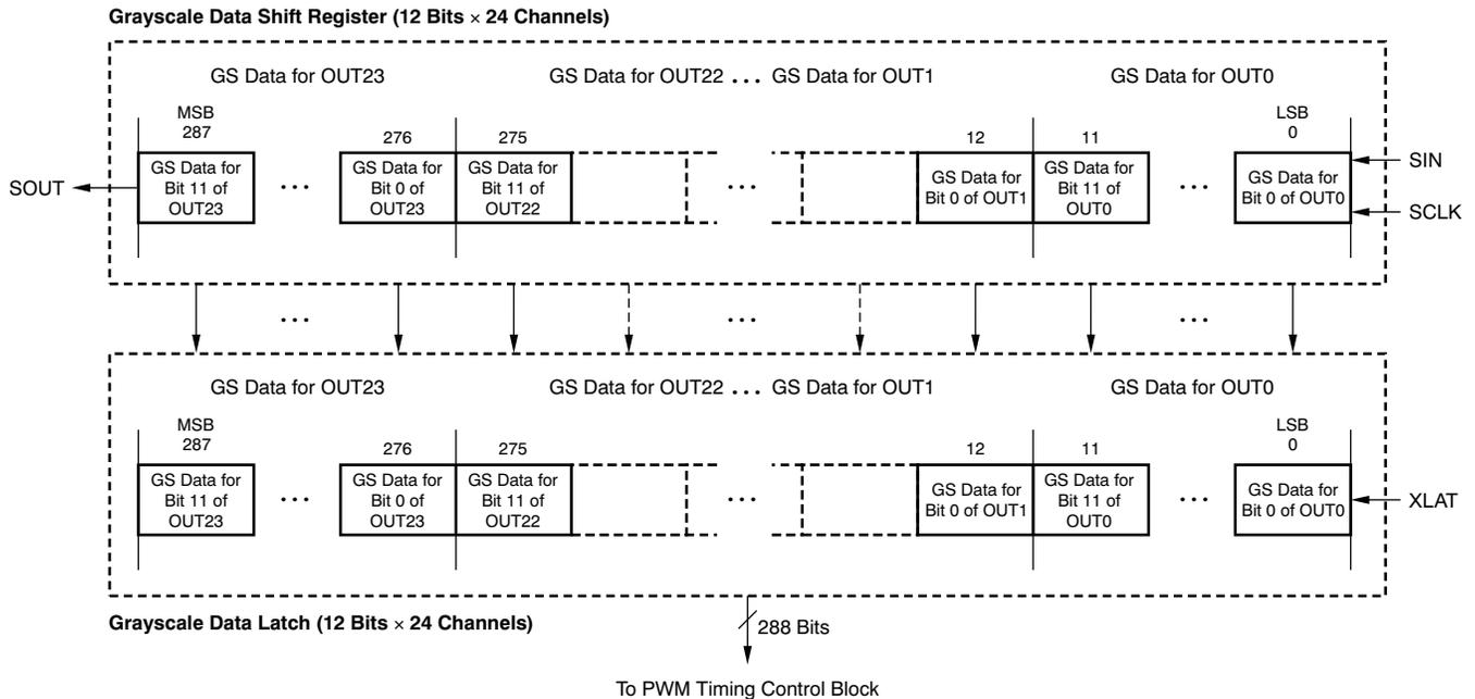
**Figure 19. Grayscale Data Shift Register and Latch Configuration**
